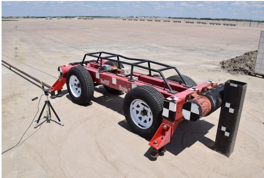
Figure 79. Rigid-Frame Bogie No. 3 and Guidance Track
